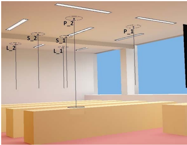
Fig. 5. The 3D view of the location of the light sensors
