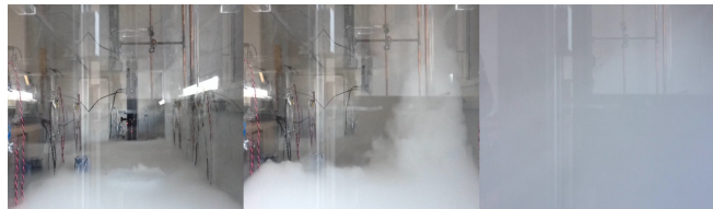
Fig. 2. Process of fog generation by dry ice sublimation.
